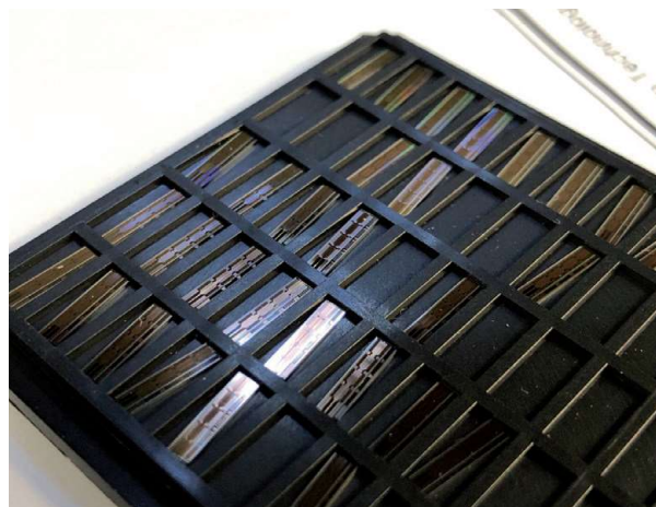
LED driver chips to control the nanoLED array
