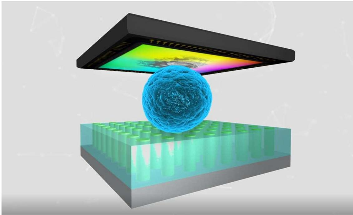
*A model of the ChipScope microscope: the specimen lying on the nanoLED surface is scanned, and the shadow image is recorded*
